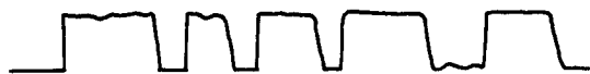
FIG. 3. Square wave as seen on the oscilloscope. Each cycle corresponds to one cycle of bubble formation.
